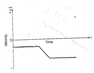
6. a car braking for a traffic light, waiting for a short time, accelerating from rest, and finally cruising at a constant velocity
